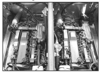
Twin 6-cyl Yanmar 6LP high rev diesel engines coupled with 241 Hamilton Jets with turbo impellers. Under 1600 hours. Cruises at 30 knots at 3500 RPM in current Bentz passenger vessel. Fuel burn: 15 gal. per hour.
