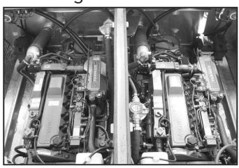
Twin 6-cyl Yanmar 6LP high rev diesel engines coupled with 241 Hamilton Jets with turbo impellers. Under 1600 hours. Cruises at 30 knots at 3500 RPM in current Bentz passenger vessel. Fuel burn: 15 gal. per hour.
